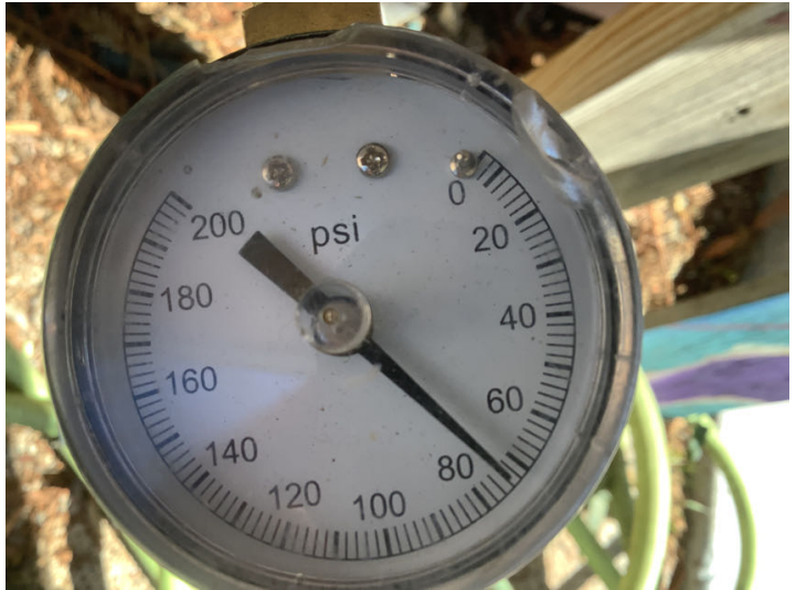
The water pressure entering the residence is under 80psi and a regulator is not required on the plumbing system.
