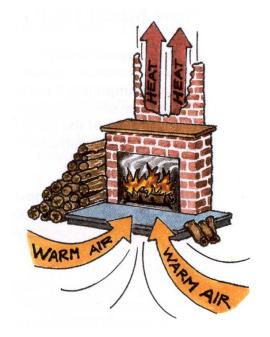
Warm air is always escaping from your house, and is replaced by unheated outdoor air. The typical house has one-half to two air exchanges per hour, and more on windy and/or very cold days. If your house has little insulation and many air leaks, you are paying to heat the outdoors. And if the outside air is smoky, soon your air inside will be too.
